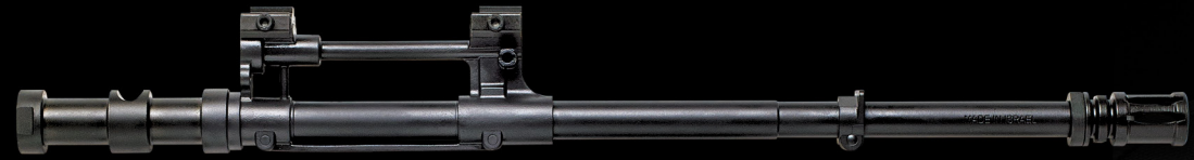
17" 9mm Luger Parabellum (9x19mm) CHF CrMoV Barrel, 1:10 RH with flash suppressor on 1/2" x 36 TPI
