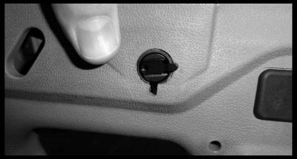
▶ Push barrel pivot lock out of the left side of rifle. Making sure that the roll pins on the barrel pivot lock line up with the slots on the body. If they are not lined up correctly they can be sheared off.
