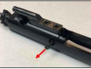
b. Tilt the bolt carrier up and remove the firing pin from the back.
