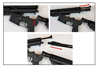
c. Pull the charging handle further to the rear then gently pull down until it drops out of the upper receiver.
