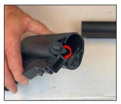
c. Pull the sleeve from the stock and remove the cap for access to the compartment. The cap is water proof, it may require a forceful twisting motion to remove the cap.
