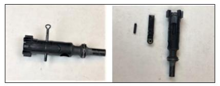
g. The bolt is now disassembled.
