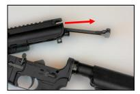
d. Push the pivot pin from left to right until the upper receiver separates from the lower receiver.
