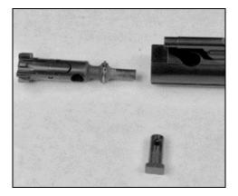
f. Place pressure on the back of the extractor and push the extractor pin through. **DO NOT REMOVE THE EXTRACTOR SPRING.**
