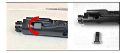
e. Pull forward on the bolt and remove it from the front of the bolt carrier.
