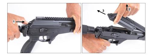
Figure 4-2: Cover Disassembly
