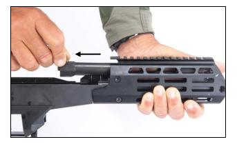
Figure 4-5: Gas Cylinder Removing
