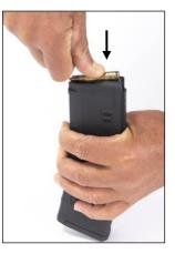
Figure 3-1: Loading the Magazine
