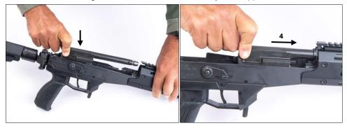
Figure 4-8: Installing the Bolt Carrier Assembly
