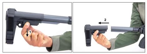
Figure 4-12: Removing the Brace
