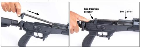
Figure 4-9: Return Spring Assembly Installing
