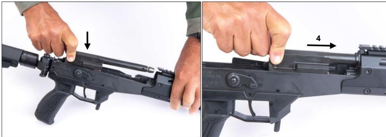
Figure 4-8: Installing the Bolt Carrier Assembly
