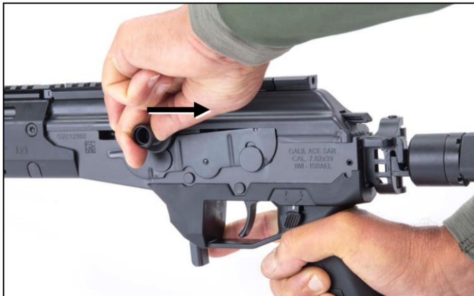
Figure 4-11: Cover Assembly (b)
