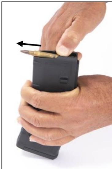
Figure 3-2: Unloading the Magazine
