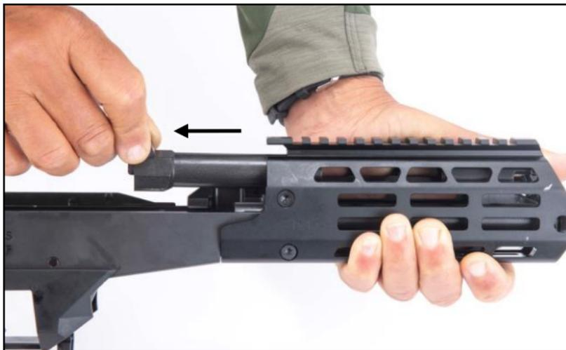
Figure 4-5: Gas Cylinder Removing
