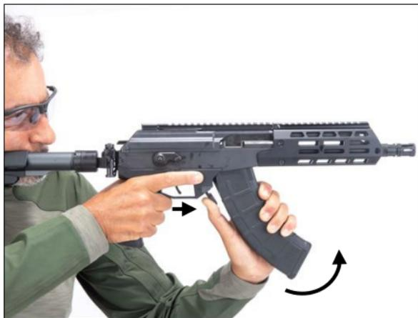
Figure 3-4: Removing the Magazine (5.45x39mm / 7.62x39mm models)
