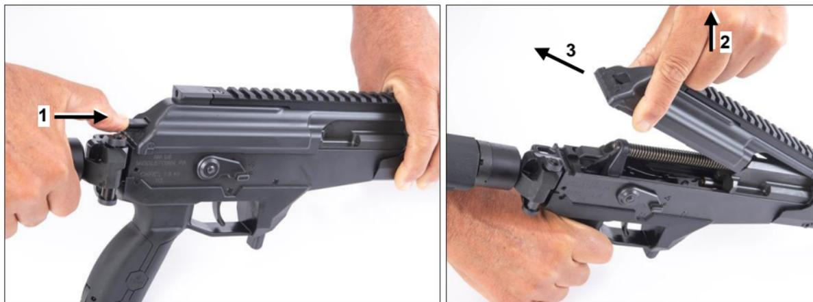
Figure 4-2: Cover Disassembly
