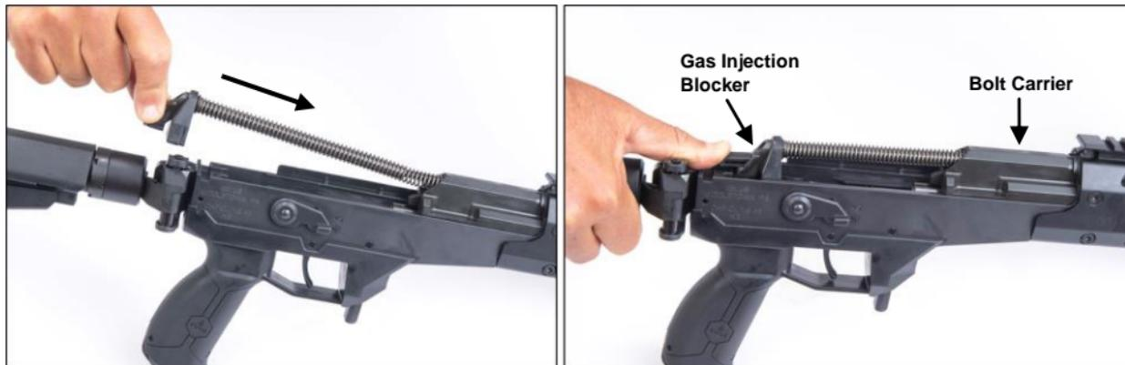
Figure 4-9: Return Spring Assembly Installing
