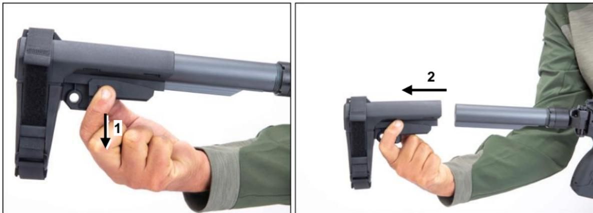
Figure 4-12: Removing the Brace
