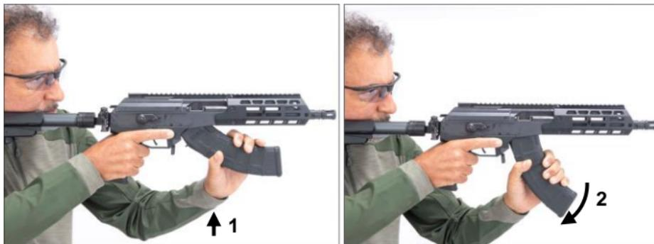
Figure 3-3: Inserting the Magazine (5.45x39mm / 7.62x39mm models)
