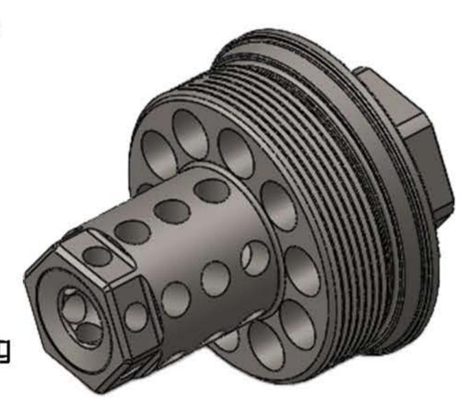
The IWI 7 silencer is a state-of-the-art reduced back-pressure solution for 7.62 NATO and 7.62mm Magnum Rifle Calibers. Built with weapons-grade nickel alloy and stainless steel components, and CNC laser-welded for durability, it withstands the demands of short barrels and full-auto firearms while maintaining the rifle's inherent precision.
