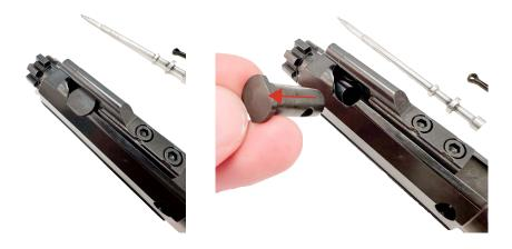
4. Pull forward on the bolt and remove it from the front of the bolt carrier.
