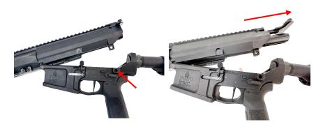
3. Pull the charging handle further to the rear then gently pull down until it drops out of the upper receiver.
