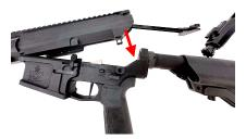
4. Push the pivot pin from left to right until the upper receiver separates from the lower receiver.
