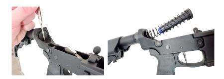
NOTE: use caution when removing, it will spring out of the receiver extension.
