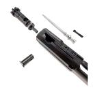
Place pressure on the back of the extractor and push the extractor pin through. DO NOT REMOVE THE EXTRACTOR SPRING.
