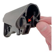
3. Pull the sleeve from the stock and remove the cap for access to the compartment. The cap is water proof, it may require a forceful twisting motion to remove the cap.
