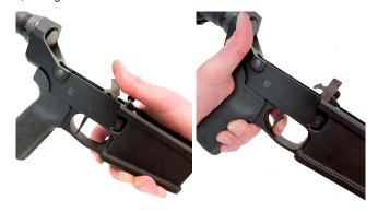
5. Ensure that the hammer is re-cocked and the safety is on before reassembly.
